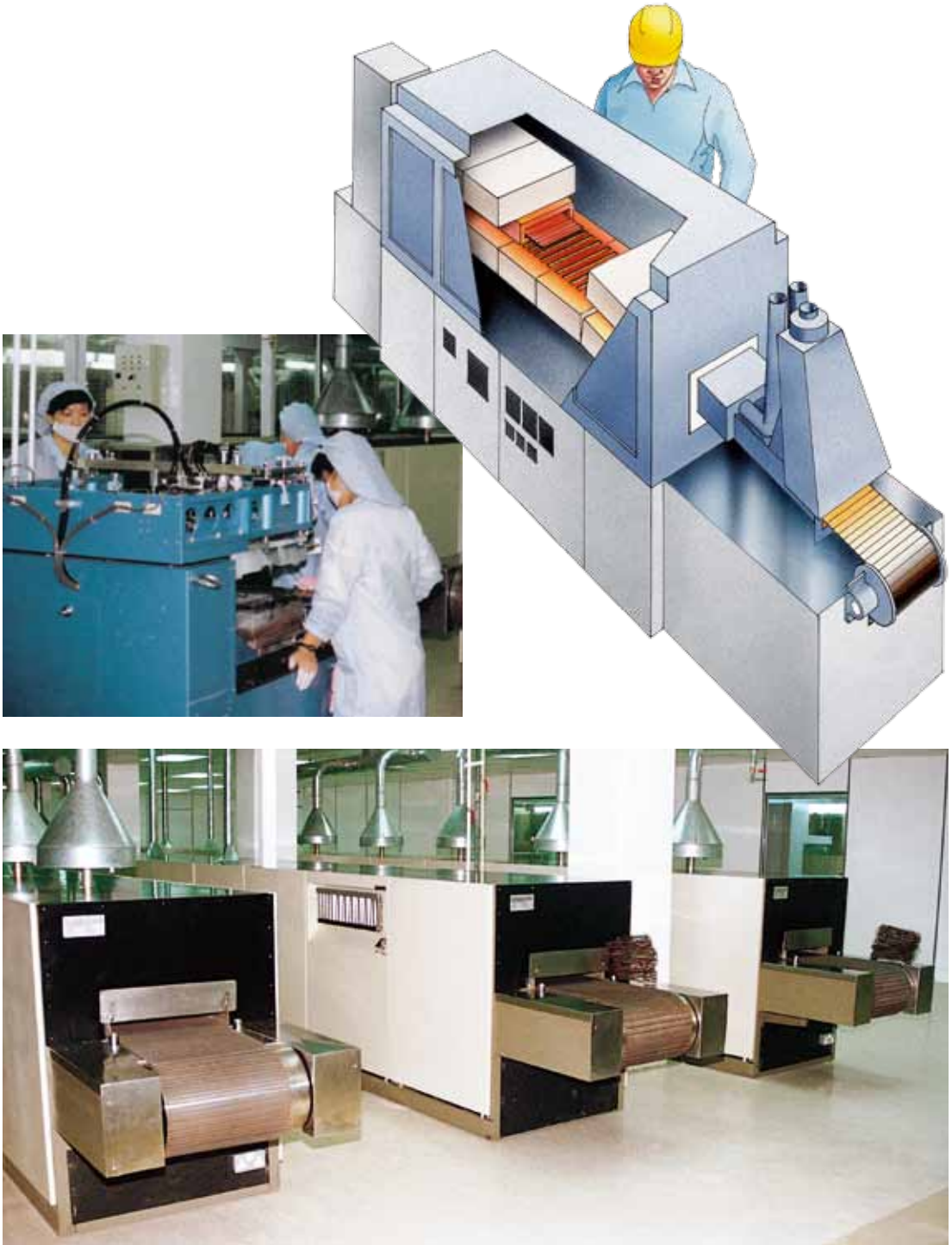
Fig. 25 Fibrothal modules used in a conveyor belt furnace.
