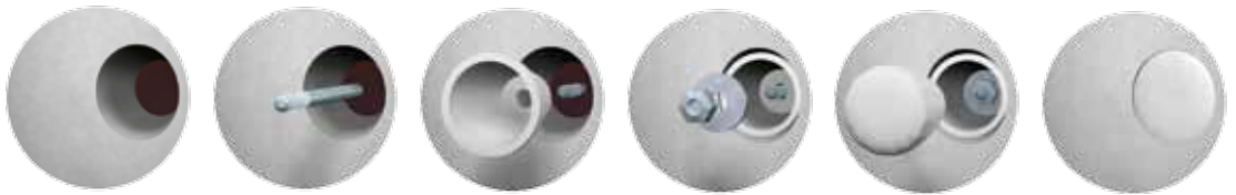
Fig. 20 Mounting of Fibrothal modules.
