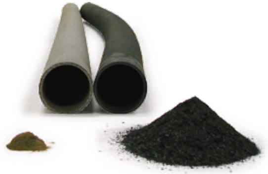
Comparison of Kanthal APMT tube versus Fe-35Ni-25Cr (after 2300 h at 1100°C (2010°F)). The FeNiCr tube is severely contaminated with oxide flakes.
