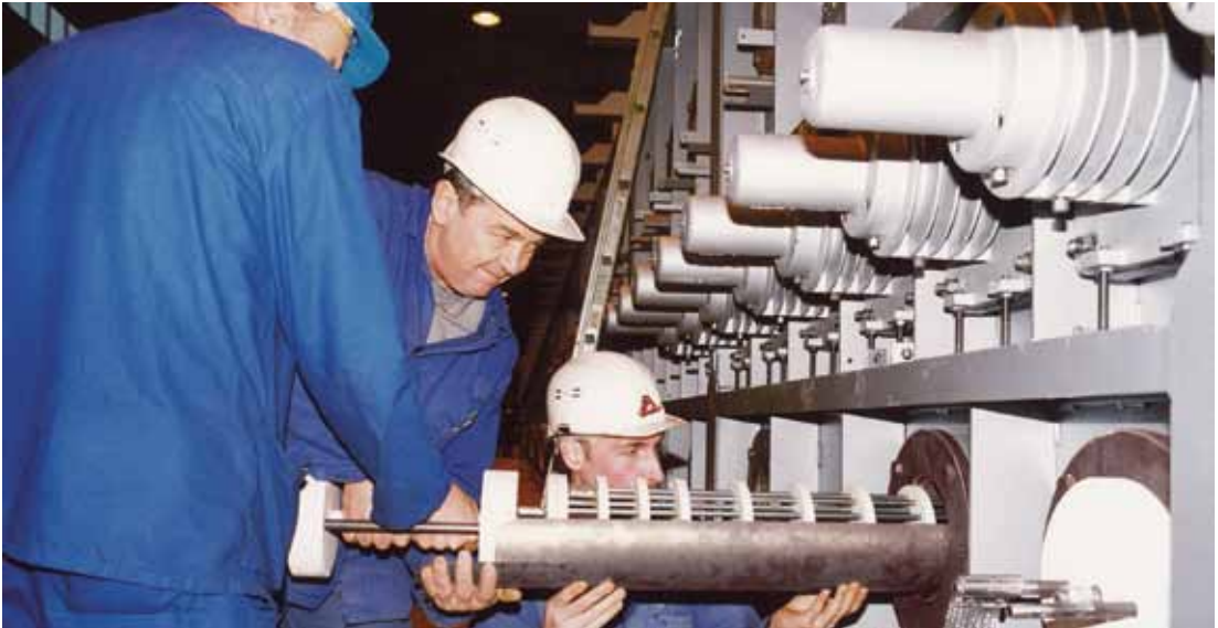
Installation of Tubothal and Kanthal APM tubes in a continuous annealing line.
