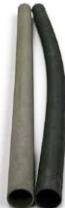
Tubes in Kanthal APMT (left) and Fe-35Ni-25Cr (right) after the sagging test.
