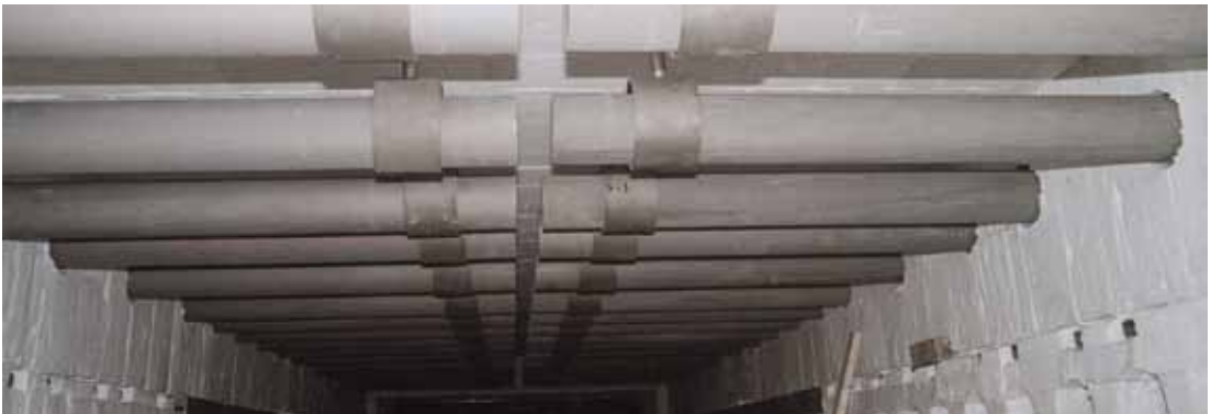
Installation of Tubothal and Kanthal APM tubes in a continuous annealing line.
