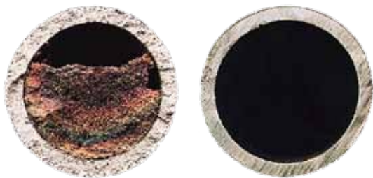
Comparison of carbon build-up in a strand annealing furnace, NiCr (left) and APM (right).
