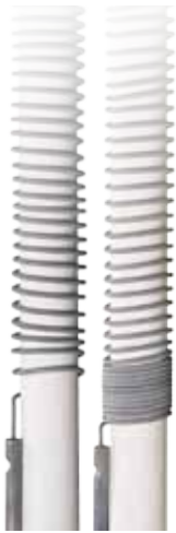
Comparison between Kanthal APM (left) and conventional FeCrAl (right) after 1250 h at max 1225°C (2240°F) element temperature.
