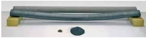
Comparison of Kanthal APMT tube vs. Fe-35Ni-25Cr (after 2300 h at 1100°C (2010°F)). The FeNiCr tube is severely contaminated with oxide flakes.
