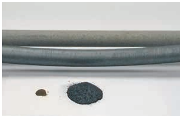
Oxide spallation. A small volume of alumina from Kanthal APMT (left) compared to the larger volume of chromia from NiCrFe (right).
